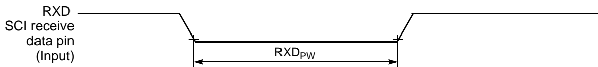
Figure 10-16 RXD Pulse Width
