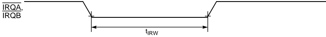
Figure 10-6 External Interrupt Timing (Negative Edge-Sensitive)
