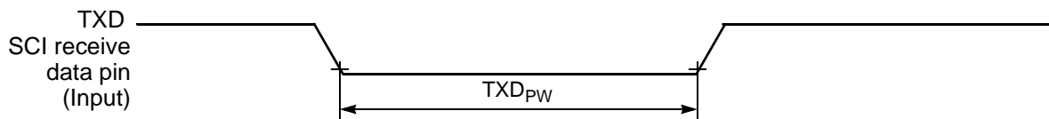
Figure 10-17 TXD Pulse Width
